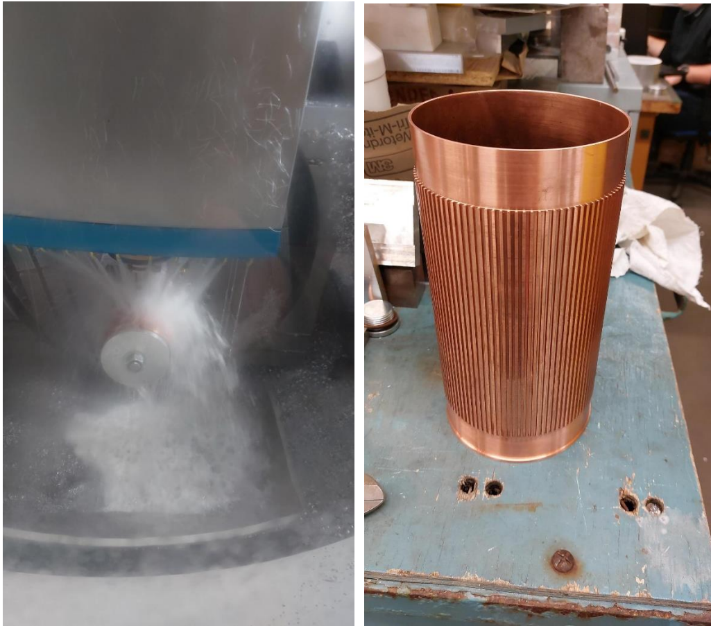
Figure 5: Copper channels being milled into the outside of the tube (left), and the finished combustion chamber wall (right).
