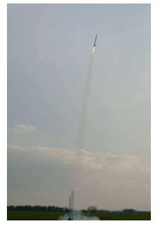
Martlet 0 reached almost 9,000ft and a maximum velocity of the speed of sound (760mph), with a motor with less than one third of the power that it was designed for. If Martlet 0 had been launched from a site with no altitude restrictions the flight would have reached around 14,000ft+ and 1400mph with a commercial 'L-class' rocket motor.
